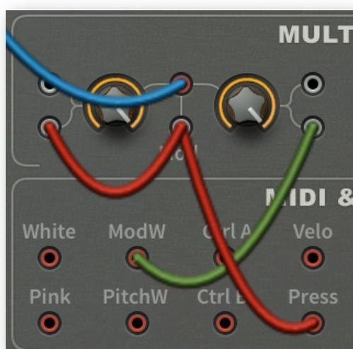
It works by using one of the two mod sources to crossfade between the other source and itself. In this example, Pressure is connected to one of the 4 regular inputs AND to the Mod socket.
