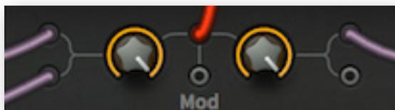
The most obvious use of a multiplex is to mix up to four signals. It acts like a regular 4-socket multiple, but with a level control for each pair... and as many outputs as you like, of course.
