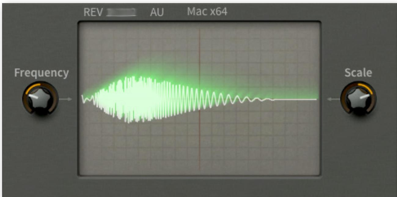
The scope displays a mono sum of the output, before the Delay effect. The *Frequency* knob on the left adjusts horizontal resolution, while the *Scale* knob on the right adjusts vertical resolution.
