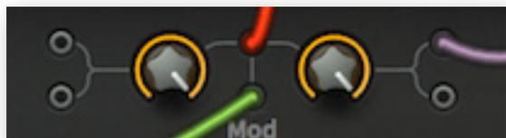
Another classic synthesizer effect like RM – use inputs 3 and 4 instead of 1 and 2. In addition to the RM sidebands, the AM output also contains the amplitude-modulated original signal. The knob on the right crossfades from the original to the AM signal.
