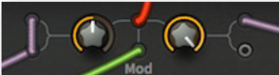
*crossfade using a bipolar modulation source*
