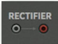
BazilleCM modules are connected together ('patched') using virtual cables. The sockets are colour-coded: inputs are grey while outputs are red – worth remembering!
