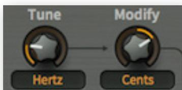
There are two types of controls: *unipolar* and *bipolar*. Unipolar knobs and sliders only allow positive values, while the *bipolar* knobs and sliders allow negative values, often within a range of -100 to +100. In the above image (the oscillator tuning controls) you can easily see that the *Tune* knob is unipolar (it starts at zero), while the *Modify* knob is bipolar. Note: while envelope sliders are unipolar, the sequencer sliders are bipolar.
