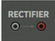
BazilleCM modules are connected together ('patched') using virtual cables. The sockets are colour-coded: inputs are grey while outputs are red – worth remembering!
