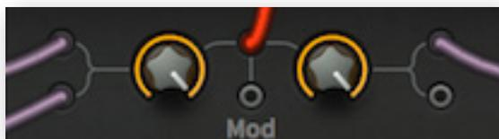
The most obvious use of a multiplex is to mix up to four signals. It acts like a regular 4-socket multiple, but with a level control for each pair... and as many outputs as you like, of course.
