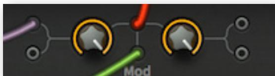
Ring modulation (as an audio effect) is traditionally used for bell-like sounds, robot voices etc.. In the above example, the signal connected to input 1 is being ring modulated (multiplied) with the signal connected to the *Mod* (modulation) input. Note: In this case, swapping the regular input signal with the *Mod* signal will make no audible difference.
