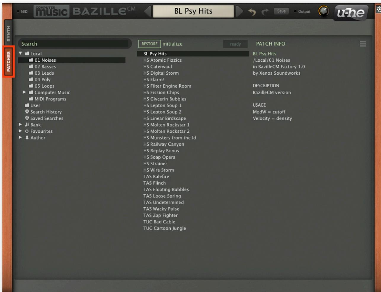
Most of the GUI is replaced by a set of three connected panels: Folders appear on the left, presets in the centre and information about the currently active preset on the right. If you can't see the folders 01 to 10, click on the triangle to the left of *Local*. If you can't see the PRESET INFO pane at all, click on the [≡] button in the top right and activate *Show Preset Info*.
