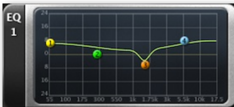
Equalizer module, bass+treble boost, dip around 1.5 kHz
