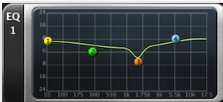
Equalizer module, bass+treble boost, dip around 1.5 kHz
